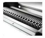
The induction-hardened solid steel cutting rollers are wear-resistant against cardboard staples and guarantee durability.
